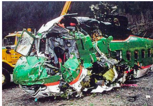
Figure 1. A Sikorsky helicopter engaged in heli-logging crashed after a freewheel disengagement.
