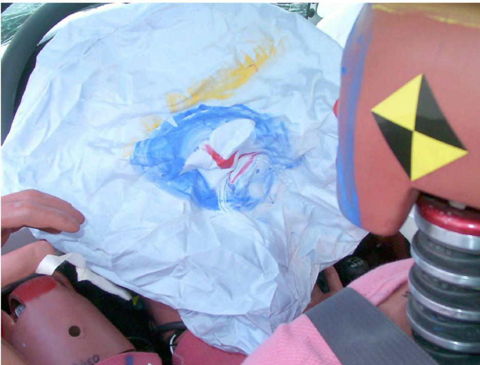
Figure 3. Chalk transfer from face of crash test dummy onto a deployed airbag during a frontal impact (source: www-nrd.nhtsa.dot.gov ).
