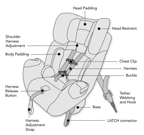
**Figure 1.** Common terminology used to describe the components of a CRS. Shown is a convertible CRS that can be used rearfacing, forward-facing and as a booster seat. Refer to the manufacturer's CRS manual for terminology related to a particular CRS.
