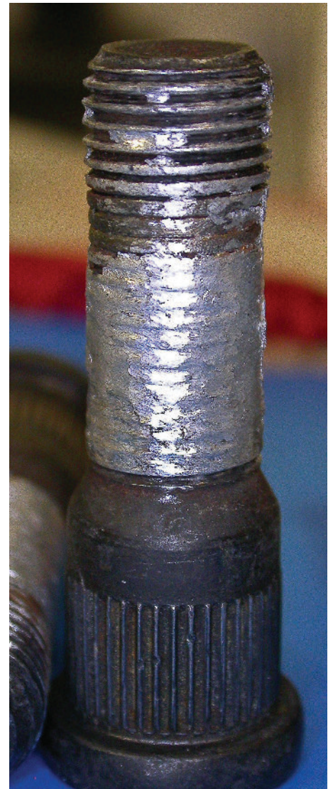
Figure 3. A heavy truck hub had a bearing failure and the consequent friction destroyed the hub and allowed it to come off the end of its axle.
